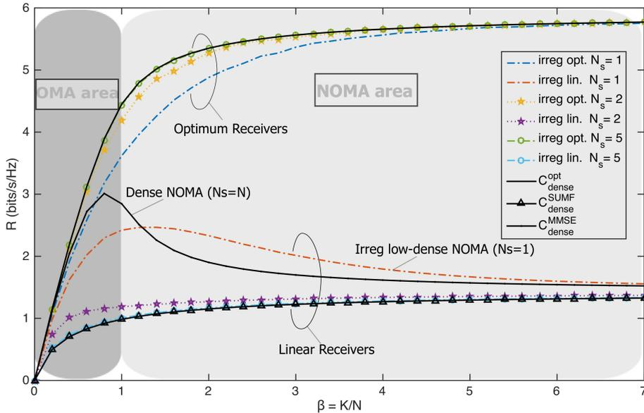
FIGURE 2: Achievable rates (bits/s/Hz) of dense NOMA vs. *irregular* low-density NOMA as a function of  $\beta$  with fixed  $E_b/N_0 = 10$  [dB] (parts of the data used to draw this figure were extracted from [23])
