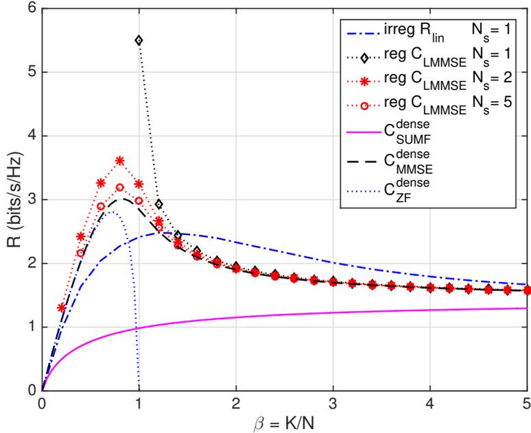
FIGURE 3: Achievable rates (bits/s/Hz) of dense NOMA ( $N_s = N$ ) with SUMF, MMSE, ZF receivers vs. low-dense NOMA ( $N_s = 1, 2, 5$ ) with linear receivers as a function of  $\beta$  for fixed  $E_b/N_0 = 10$  [dB]
