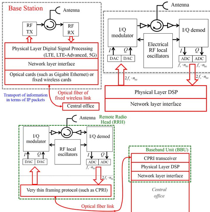
**Fig. 2** Comparison between traditional backhauling and new DRoF fronthauling: simplified schematics. Top left: traditional backhauling architecture. Top right: zooming in the RF and BBU parts of the traditional architecture. Bottom: DRoF fronthauling architecture
