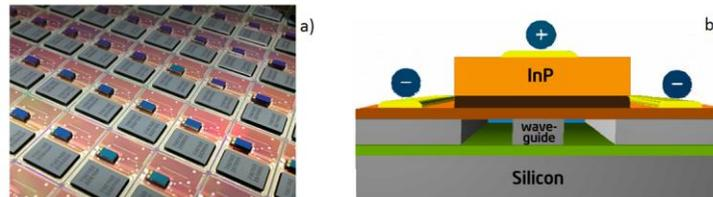
The integration of lasers and optical amplifiers is also possible by heterogeneous integration of Silicon photonics and III-V semiconductor technologies. The hybrid integration of III-V semiconductor optoelectronic components onto Silicon photonics PICs can be obtained in different ways, as for example flip-chip integration, hetero-epitaxial growth, wafer bonding or transfer printing.
