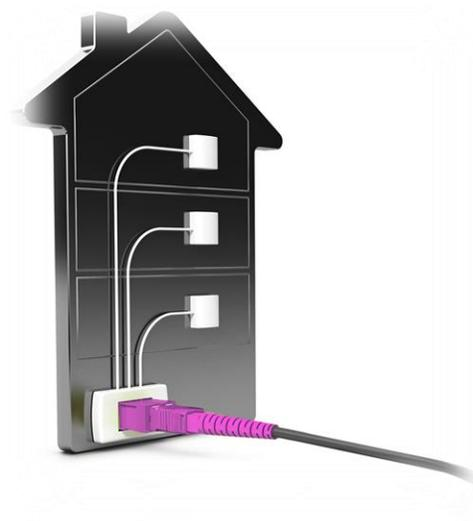
**Open Fiber's ultra-fast network** is built using **Fiber To The Home (FTTH)** technology, meaning the entire connection from the exchange to the customer's home is in optical fiber. This provides maximum performance with **speeds of up to 10 Gigabit per second (Gbps)**.
